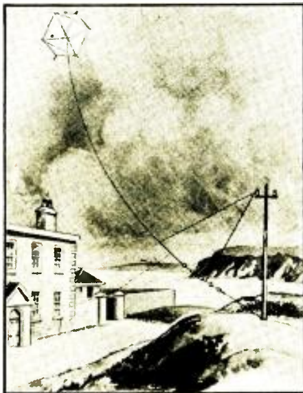
A reconstruction of the kite used by Marconi in receiving the signals from England. This was an emergency aerial which replaced the large aerial blown down by a gale.
